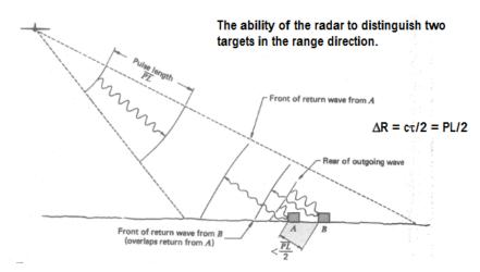
Fig 1. Range resolution is dependent on pulse length
